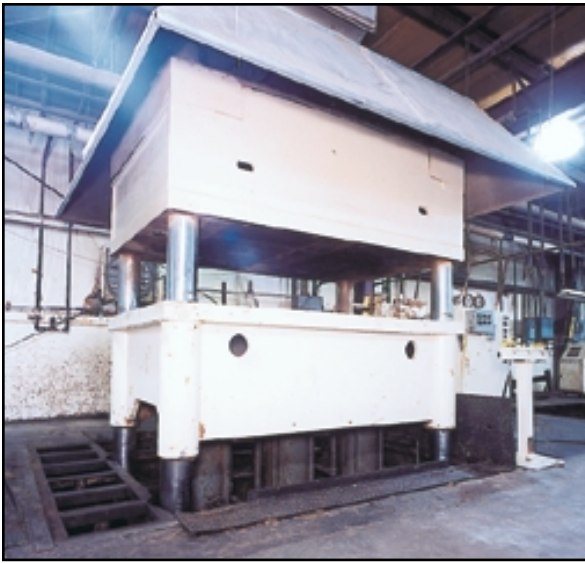
ST. LAWRENCE 600-TON 3-POINT UP-ACTING 4-POST HYDRAULIC PRESS
