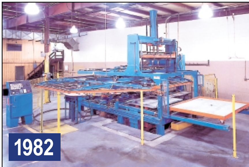
BROWN MODEL R224 72" X 96" CAPACITY 4-STATION ROTARY VACUUM THERMOFORMING MACHINE
