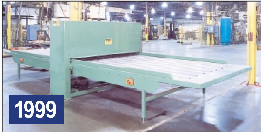
CORRUGATED CONVERTING EQUIPMENT MODEL DC80 80"W CAPACITY PINCH ROLLER-TYPE DIE CUTTING PRESS
