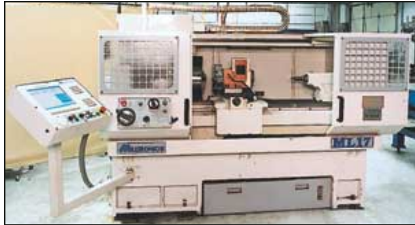
MILLTRONICS MODEL ML17 17" X 36" FLATBED CNC LATHE
