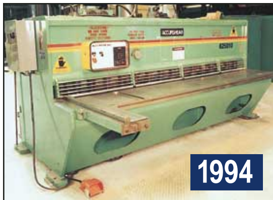
ACCURSHEAR MODEL 625010 10' X 1/4" HYDRAULIC SQUARING SHEAR
