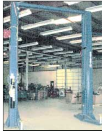
1 OF 6 ROTARY 15,000-LB. CAP. 2-POST AUTOMOTIVE LIFTS
