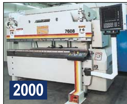
ACCURPRESS MODEL 7608 60-TON X 8' HYDRAULIC PRESS BRAKE
