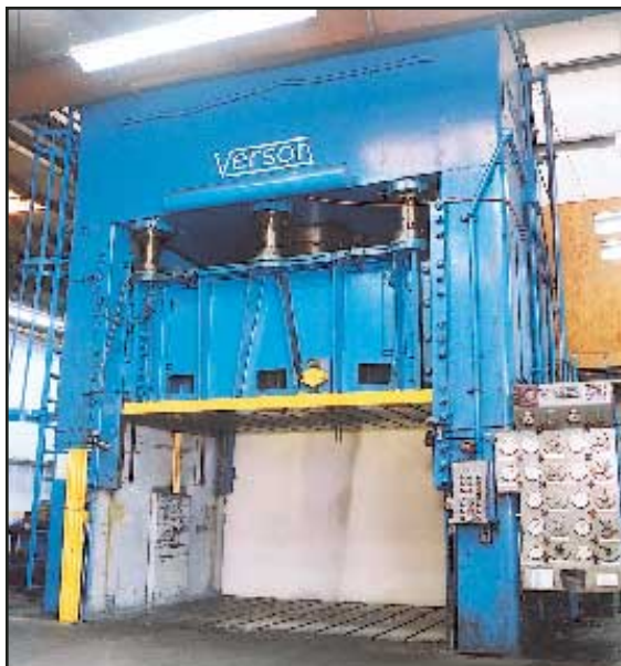
VERSON MODEL 1600-HD-1D-144T 1600-TON TRIPLE-ACTION HYDRAULIC STRAIGHT SIDE PRESS
