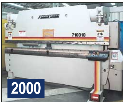
ACCURPRESS MODEL 710010 100-TON X 10' HYDRAULIC PRESS BRAKE
