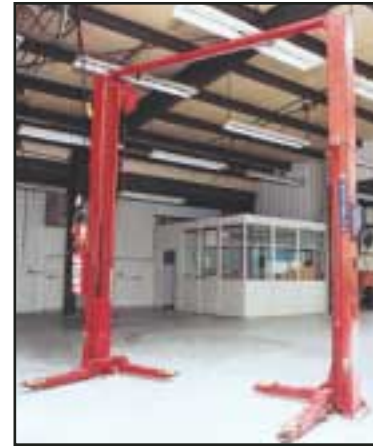
1 OF 55 ROTARY 9000-LB. CAP. 2-POST AUTOMOTIVE LIFTS
