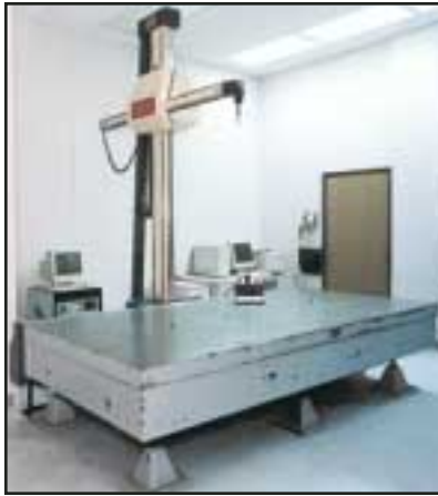
MORA CANTILEVER-TYPE COORDINATE MEASURING MACHINE
