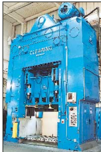
CLEARING D2-400-250-84-42 650-TON DOUBLE-ACTION S.S. PRESS
