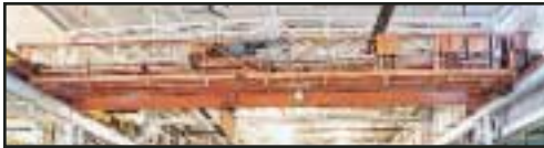
MILWAUKEE CRANE 10-TON CAP. DOUBLE GIRDER TOP RUNNING BRIDGE CRANE
