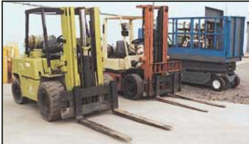
PARTIAL VIEW OF FORKLIFTS AND SCISSOR-LIFT AERIAL WORK PLATFORMS
