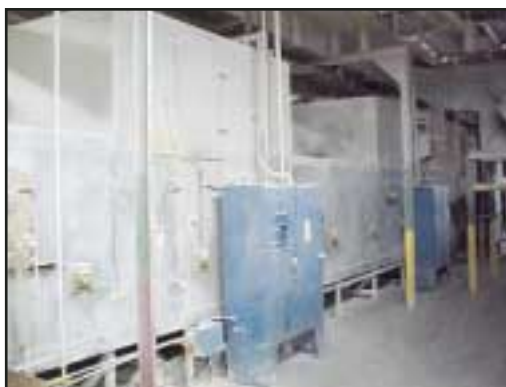
SANDVIK 72" X 200' 8-ZONE CONTINUOUS ELECTRIC CURING OVEN
