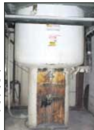
DAY DAYMAX MODEL 1000 850-GALLON HIGH SHEAR DISPERSION BLENDER
