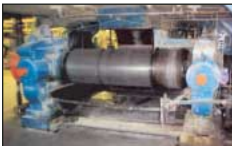
EEMCO 26" X 84" 200-HP 2-ROLL UNI-DRIVE RUBBER MILL
