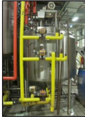
1999: Feldmeier 4911 1000L Stainless Steel Jacketed Vacuum Mixing Tank
