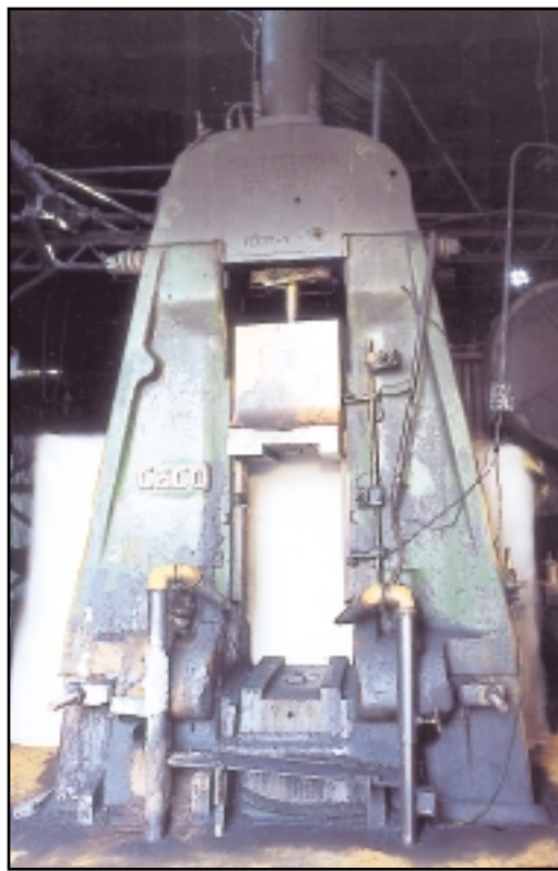
1 OF 2 CHAMBERSBURG CECO-DROP 3000-LB. CAPACITY AIR DROP HAMMERS
