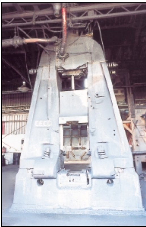
1 OF 2 CHAMBERSBURG CECO-DROP 40-CDE 4000-LB. CAPACITY AIR DROP HAMMERS
